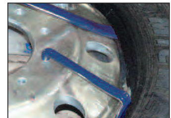
• Curved end For mounting and demounting top bead
